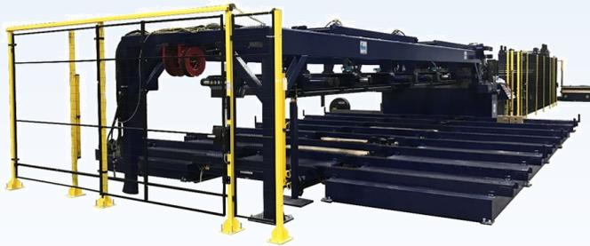
with Pallet Staging. What is unique to this line is the ability to stack up to 338" blanks, and longer blanks will process with end discharge as needed for future manufacturing needs of the customer. Added to the Morgan Olson facility in late February was our 20,000 lb. Upender to allow coils that are delivered eye-to-the-sky to be oriented for loading onto the Cut-to-Length System.
