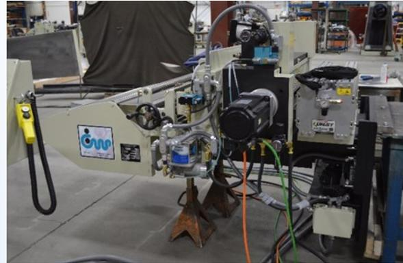
The line includes a 20,000 lb. capacity uncoiler with secondary coil clamping arm for safe thread-up of high yield materials, automatic brake tension control, and coil loading car.
